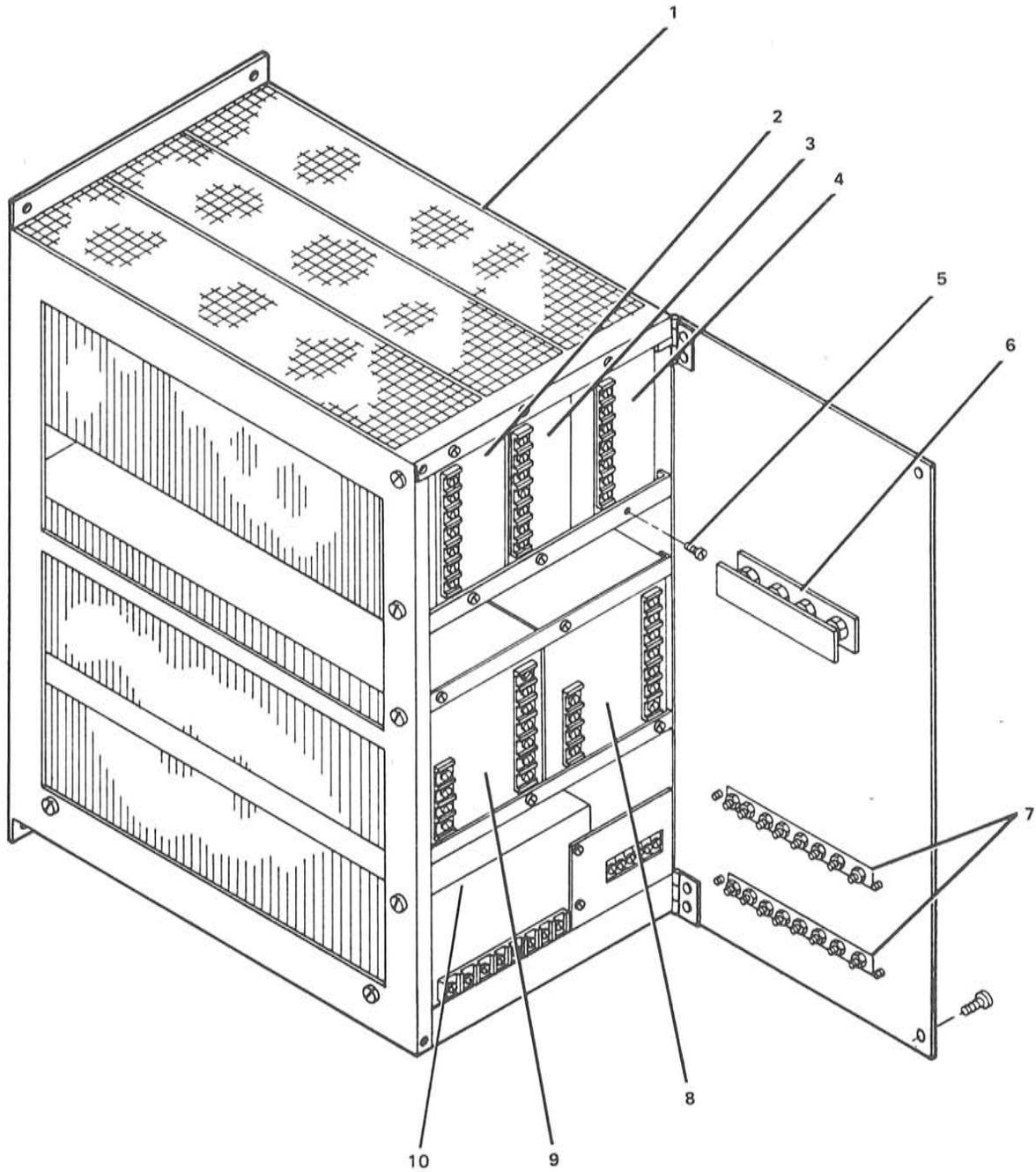
FIGURE 14. D.C. POWER SUPPLY ASSEMBLY. SEE LIST 14.
