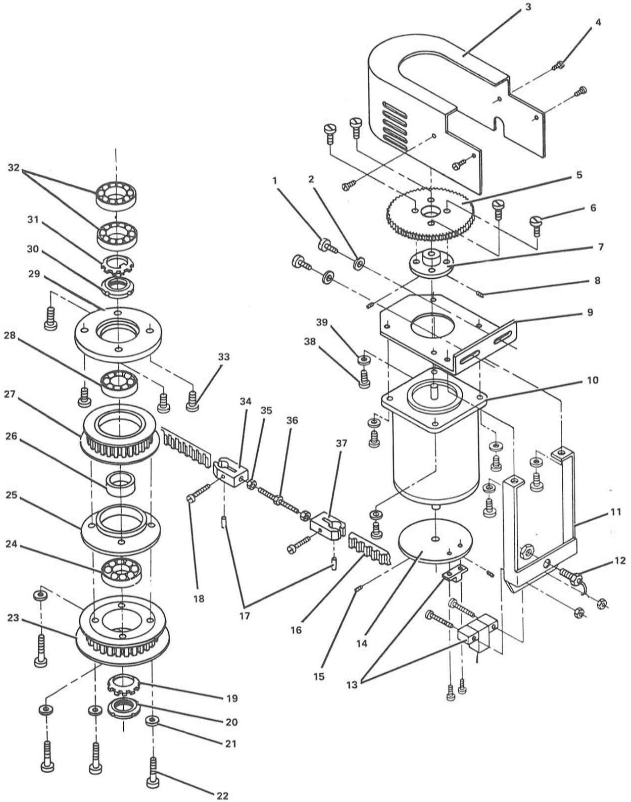
FIGURE 6. ROLL MOTOR AND DRIVE ASSEMBLY. SEE LIST 6.
