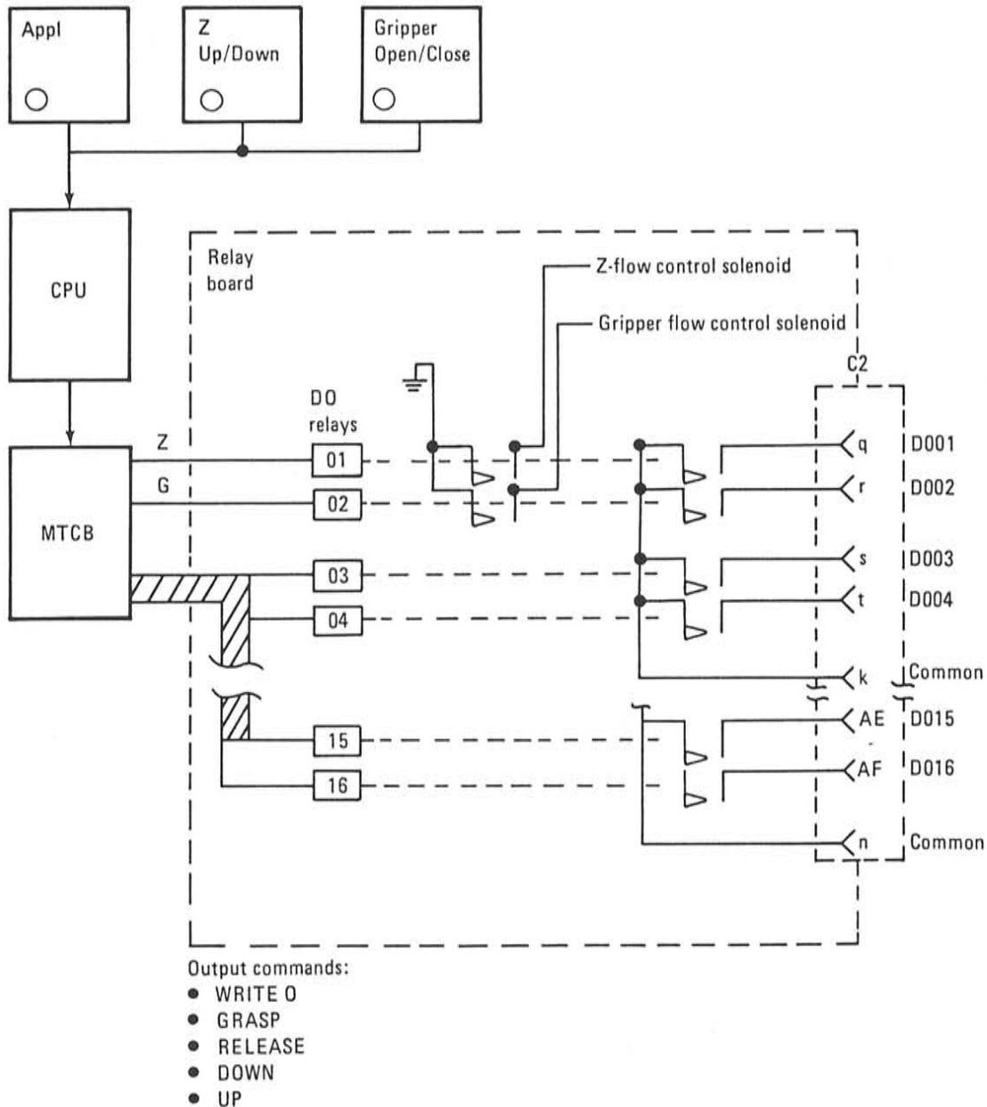
**Note:** The relays for activating the Z and gripper solenoids have two normally-open contacts each. One contact activates the solenoid and the other the user DO point. Refer to "Section 11 - Wiring Diagrams" for detailed wiring of the DO relay points.
