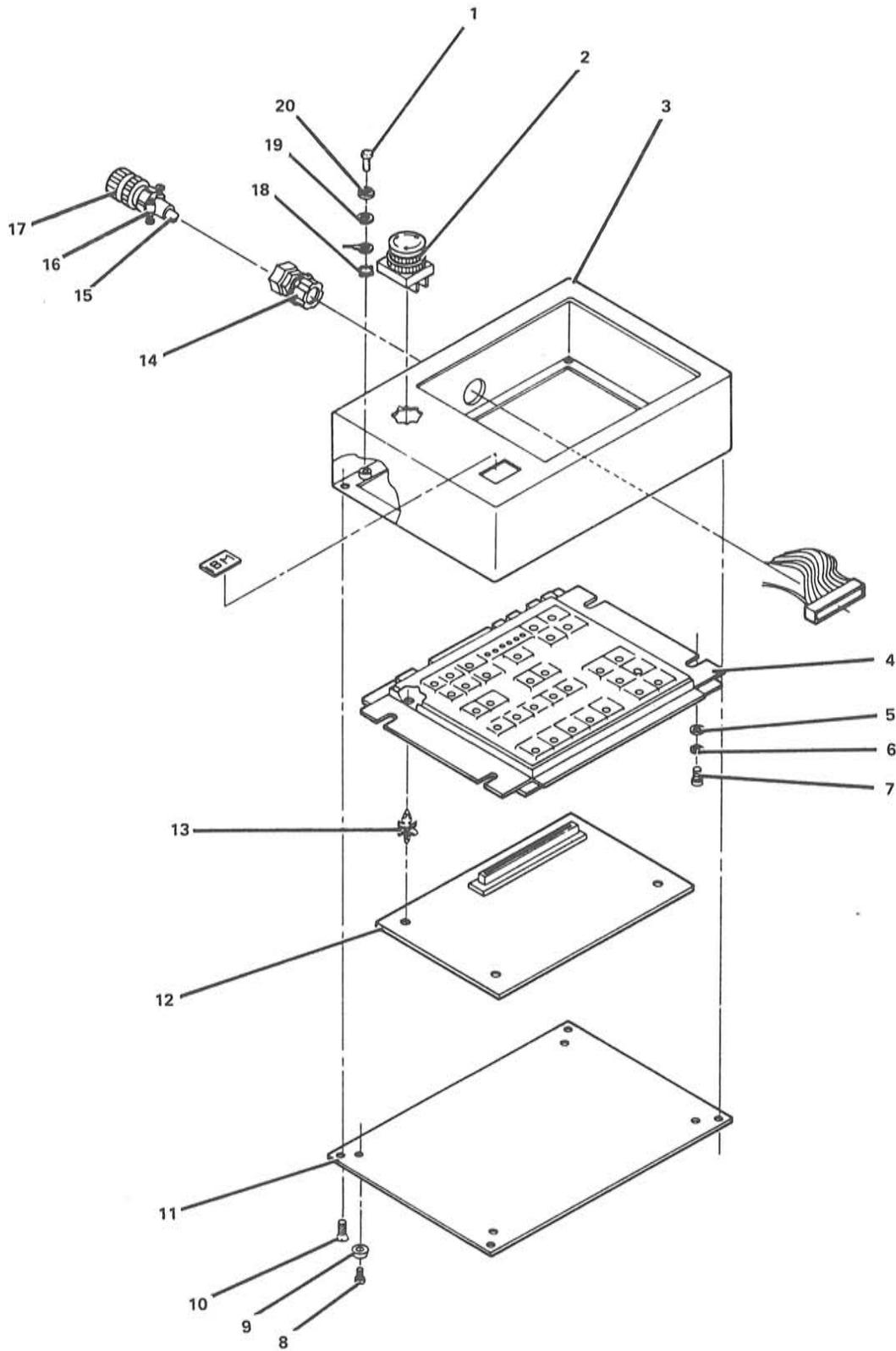
FIGURE 8. CONTROL PANEL ASSEMBLY. SEE LIST 8.
