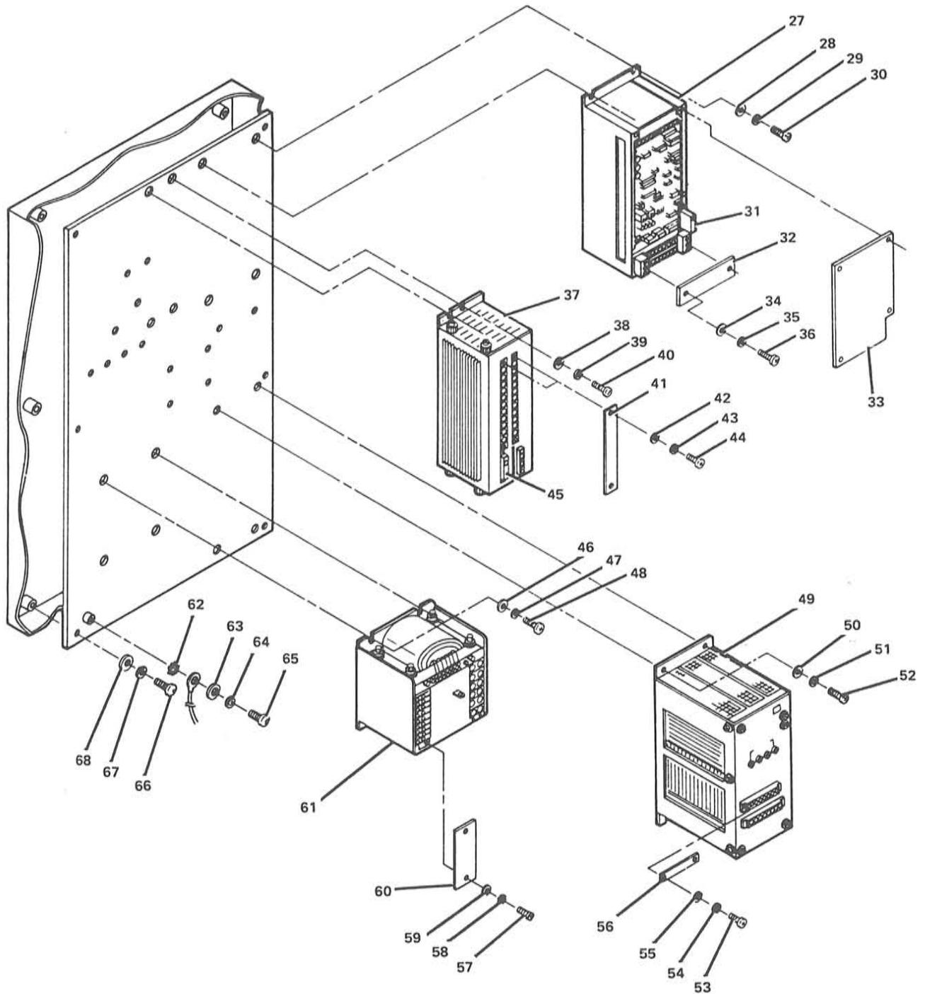
FIGURE 11. BACK PANEL. SHEET 2 OF 2. INDEX NOS. 27-68. SEE LIST 11.
