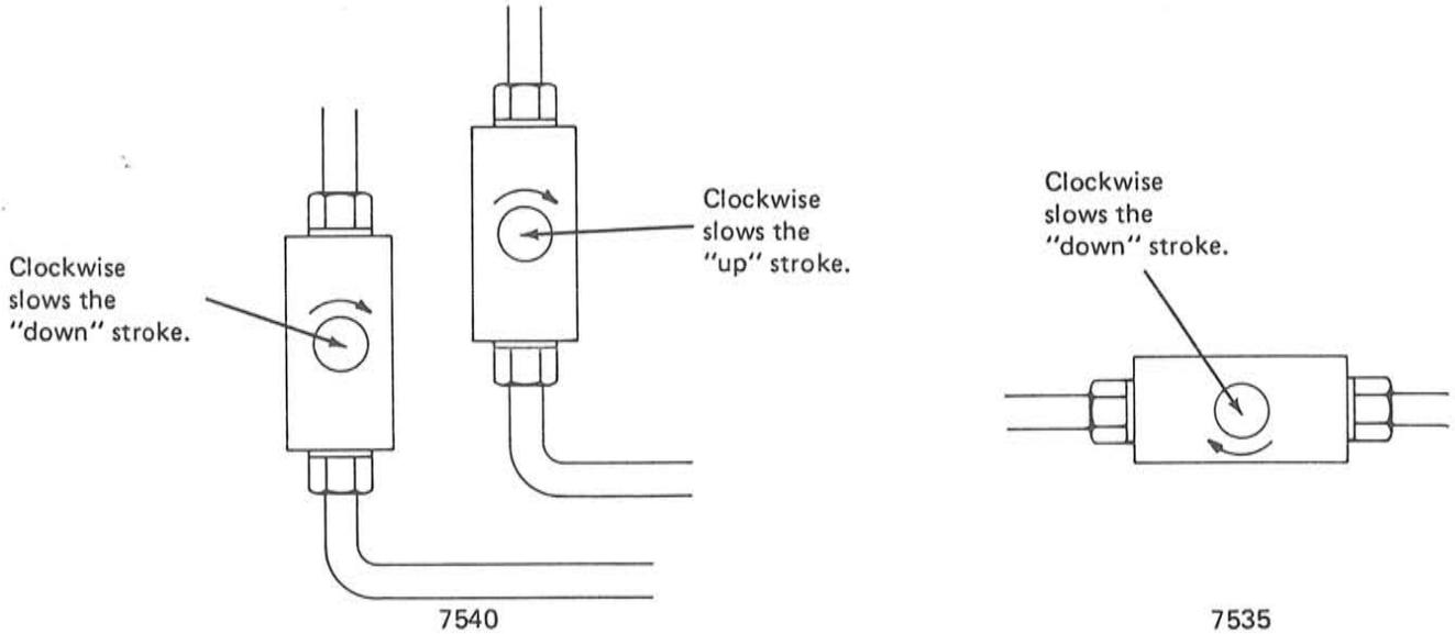
The 7540 has an air cushion adjustment for the end of stroke. Adjust as shown below:
