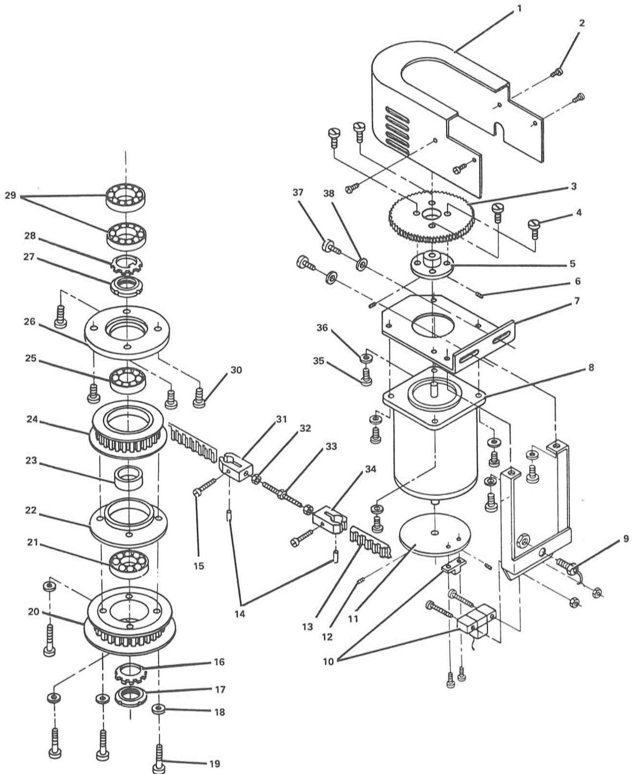
FIGURE 6. ROLL MOTOR AND DRIVE ASSEMBLY. SEE LIST 6.
