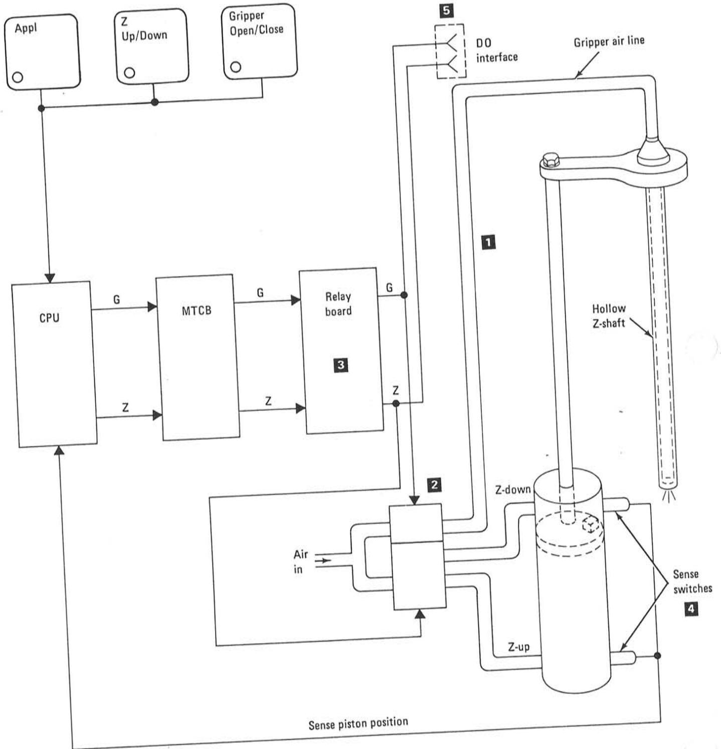
1. The Z-shaft is driven by an air cylinder that is connected to a flow control valve.
