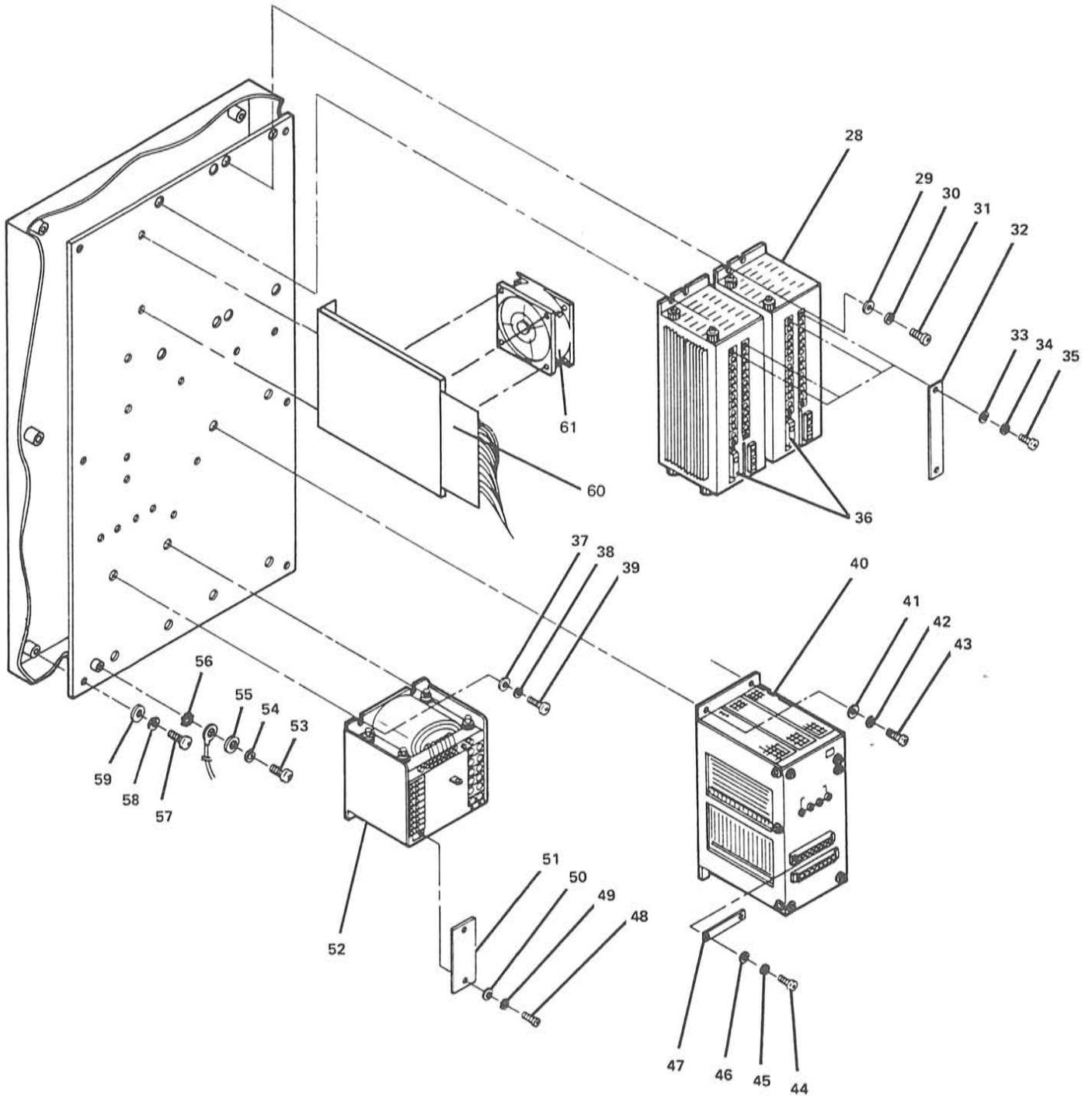
FIGURE 11. BACK PANEL. SHEET 2 OF 2. INDEX NOS. 28-59. SEE LIST 11.
