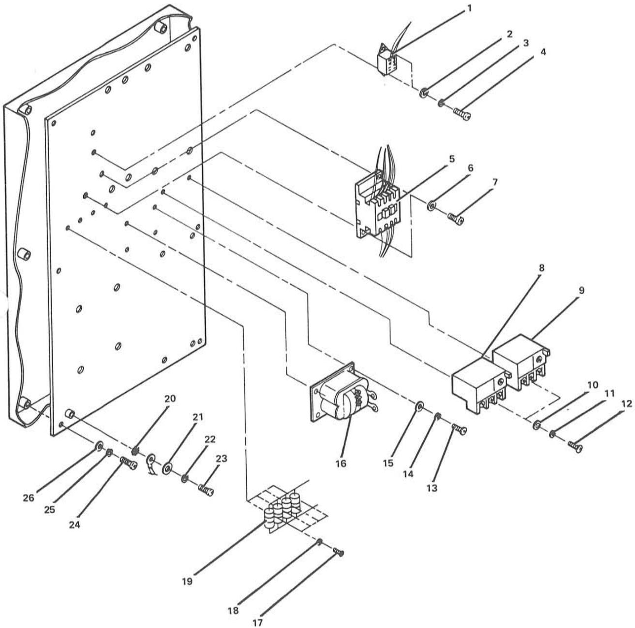
FIGURE 11. BACK PANEL. SHEET 1 OF 2. INDEX NOS. 1-26. SEE LIST 11.
