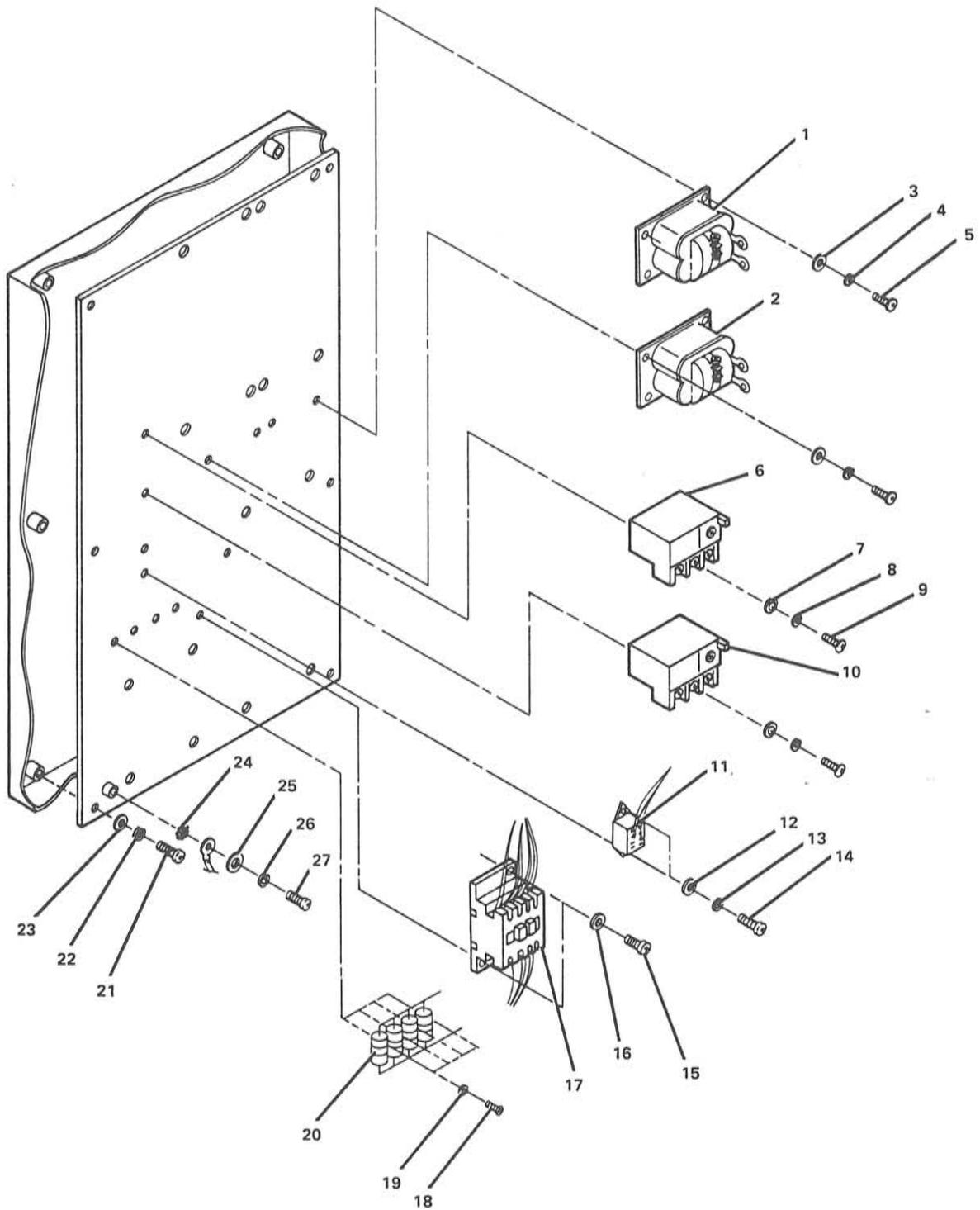
FIGURE 11. BACK PANEL. SHEET 1 OF 2. INDEX NOS. 1-27. SEE LIST 11.
